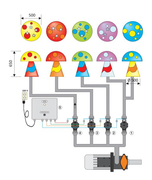
The spouters in the colourful mushrooms are regulated separately with a control unit and electrical valves. The control unit (5) and the valves (1 till 4) are included. Not included: the pump and the pipe work.
