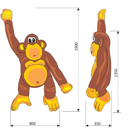
Very suitable to combine with the wall decoration jungle (9925). On request the monkey is available in a water spouting version. In that case you will need a water supply of Ø 32 mm. Than the place of the spout nozzle will be in its mouth.
