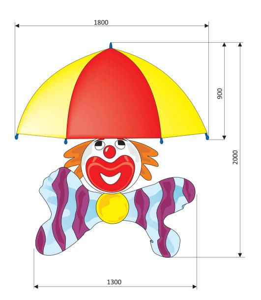
Water spouting relief in the shape of a clown with an umbrella, to be fixed to a wall. 4 Nozzles on the clown's head are standard. Several other spouting options are possible. For example as a shower. In that case we will build in showerheads.
