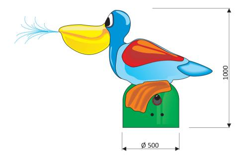
The pelican has a built in hand pump. If the water depth is more than 350 mm, the pelican needs a base (9907). The pelican is also available as a spouting object without hand pump (9802b).
