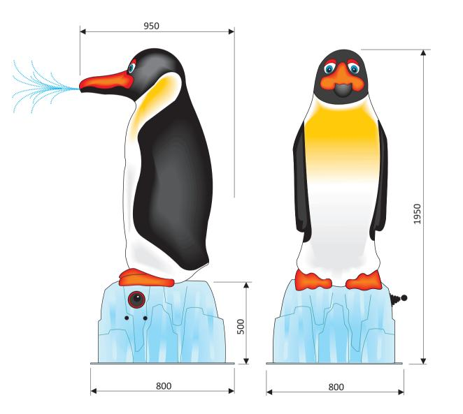
The penguin has a built in hand pump. If the water depth is more than 450 mm, the penguin needs a base (9907). The penguin is also available as a spouting object without hand pump (9803b).
