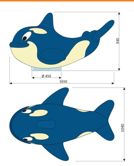
The orca can be placed in a pool with a water depth of 250 mm. In case of a higher water depth the orca should be mounted on a base.
