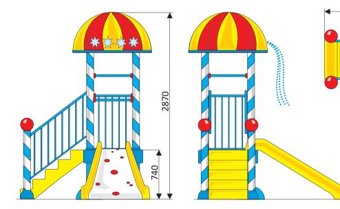
If there is a water supply the slide can spout water from the cap. Standard: water spouting continuously. Optional: the hut can be provided with a push button or handle. The stair steps have a non-skid finish.
